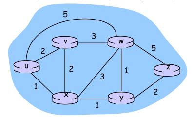
3. List changing processes of three tables of node X, Y and Z with the distance vector algorithm, from the time before the X-Y link cost is changed from 4 to 1 to the time three tables are stabilized. (第 1 行 table 是未變動前的穩定狀況,後 3 行 table 一行 3% (x, y, z 各看自己那列 1%),共 9%。數值有變動時,要寫出公式,各 1%共 4% => total 13%)
